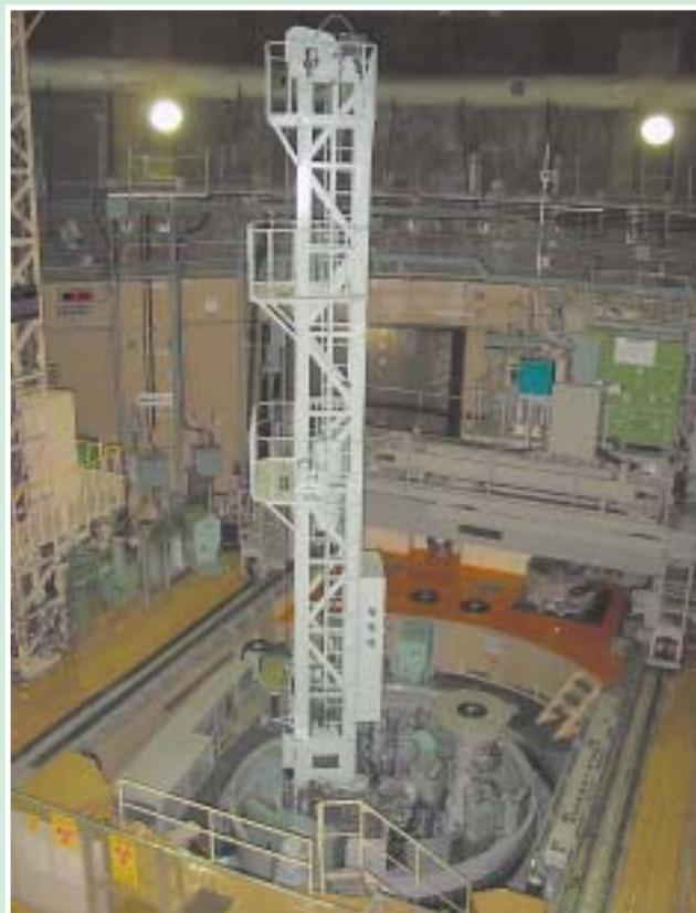
Head of the experimental fast reactor "Joyo" to which the fuel handling machine has been attached.
